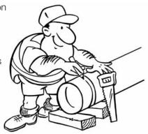
I measure the pipe socket inside and subtract 5mm to make it shorter. This is the witness mark
