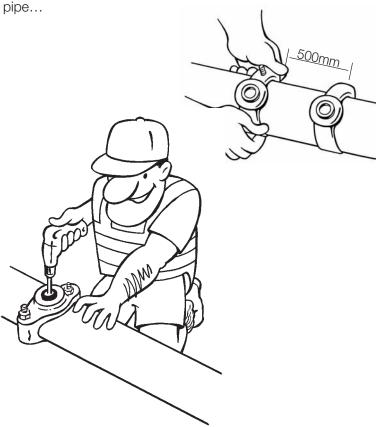
Never ever use a flat/spade bit or twist drill bit on PVC pipe! That got ya didn't it... Yeh it got me too! I found out the hard way. I now use a **sharp** fine tooth hole saw - it never lets me down! (Make sure it stays sharp!)
