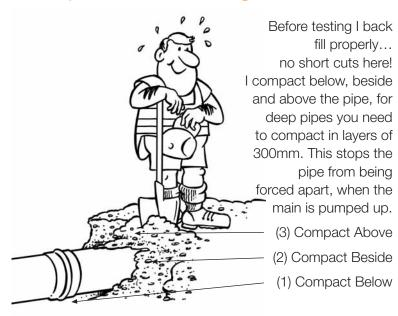
I backfill with solid material like sand, mixed sized crushed pea metal or scoria which has no large (over 20mm) stones in it. I must fill all the gaps and spaces in between the pipe & trench. Once the metal is placed I haunch the bottom of the side support zone by shuffling my shovel along the pipe. This shuffles metal under and beneath + into the 5 o'clock to 7 o'clock zones.
