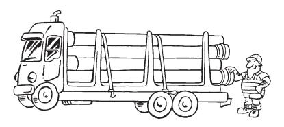
Y'know – you've got to look after these PVC pipes. They must NOT roll around the truck deck and the socket ends must stick out and be protected to avoid damage.
