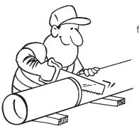
I always cut pipe using a fine-tooth hand saw, it's much easier with blocks of wood under each pipe. Y 'can use a petrol power saw with an abrasive disk too.
